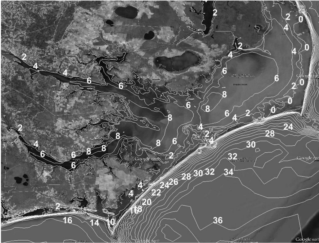
Figure 2.12 Contours of Significant Wave Height (ft) during Hurricane Ione.
